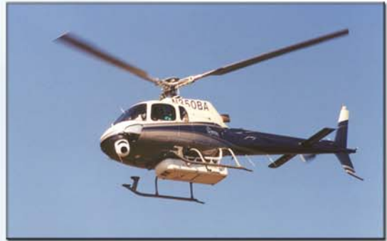
One of Aerotec's two AS350 helicopters, equipped with the Saab TopEye lidar survey system, video cameras, and black-and-white camera
